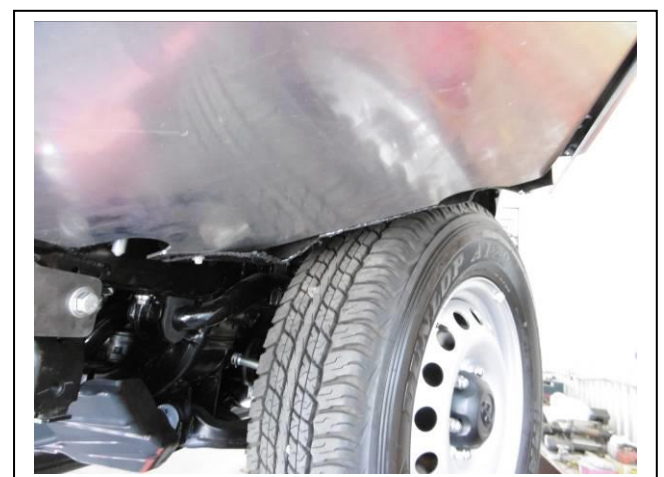
Figure 20. Liner trimmed to fit
